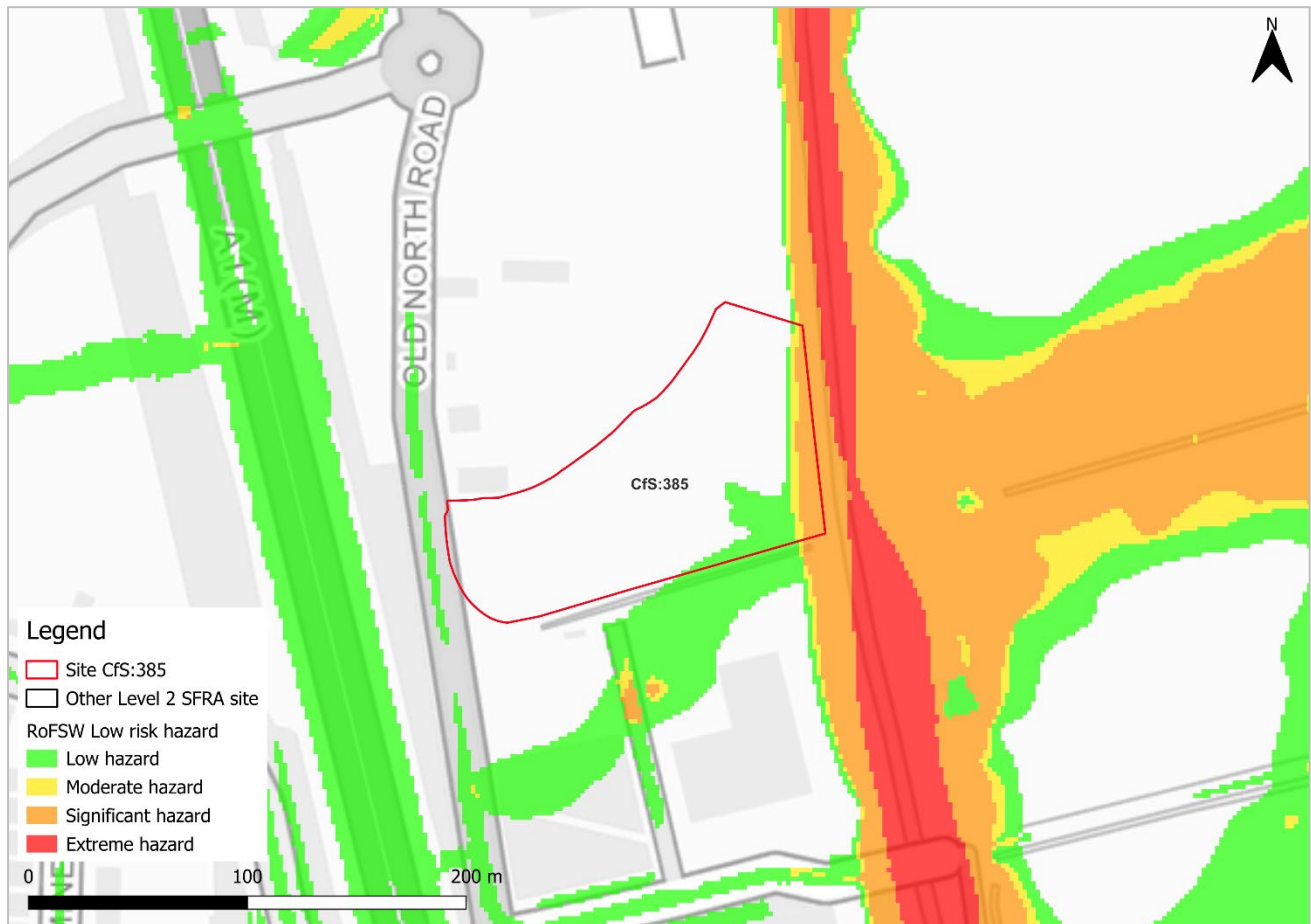
Figure 3-3: Low risk event surface water flood hazard 1 (Third generation - Risk of Flooding from Surface Water map)
