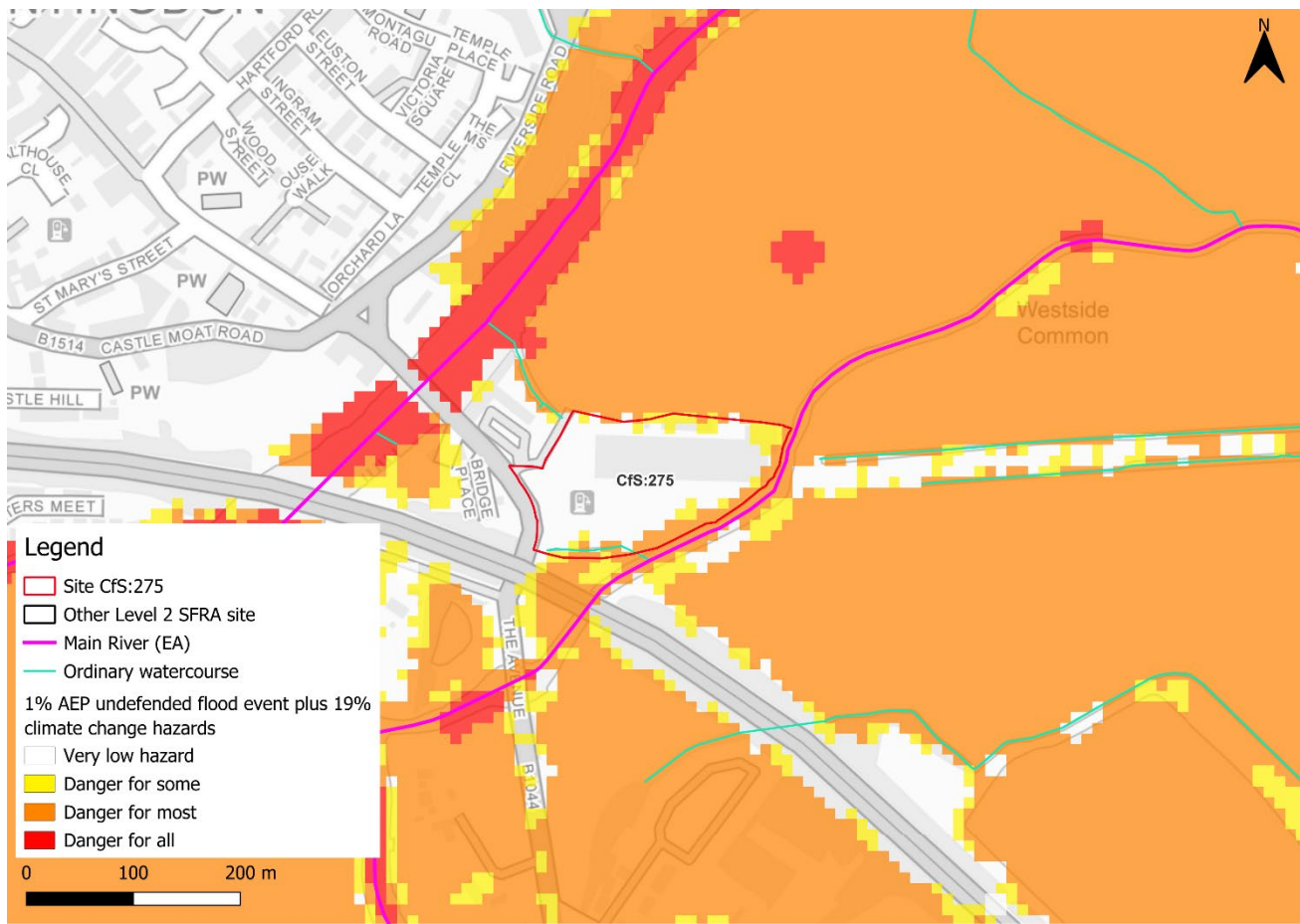
Figure 2-8: Flood hazard 1 for 1% AEP undefended flood event +19% (central climate change allowance)
