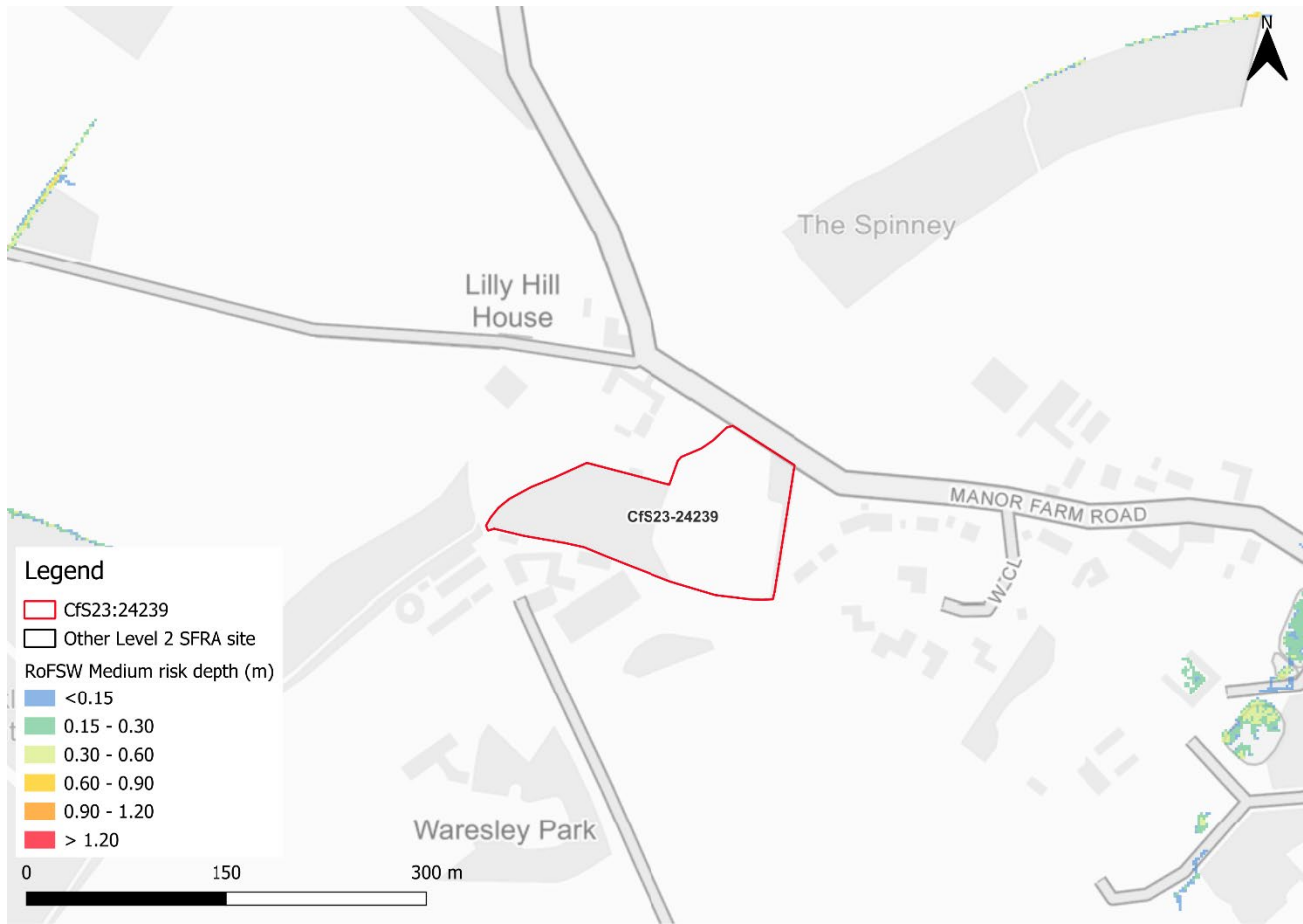
Figure 2-17: Medium risk event surface water flood depths (Third generation - Risk of Flooding from Surface Water map) within CfS23:24239
