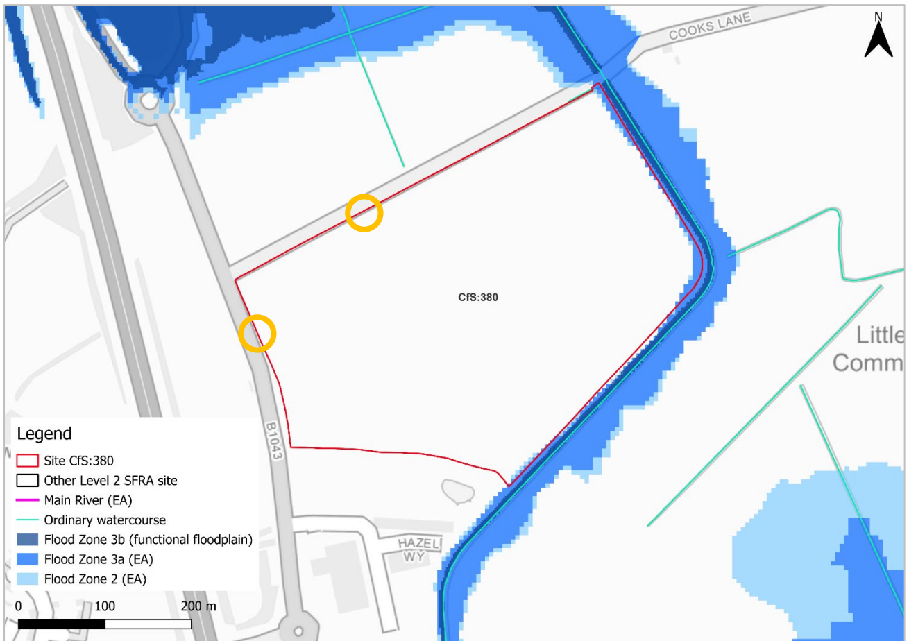
Figure 2-5: Potential access and escape route
