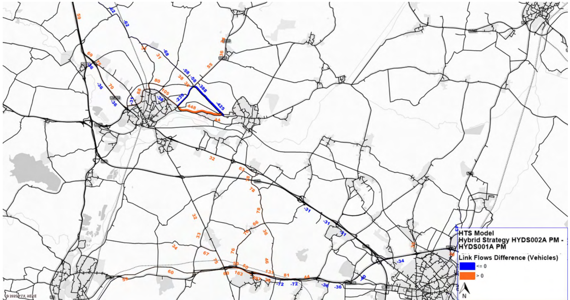
Figure C-9 - Difference in link flow between the DS and DS with EWR – PM period
