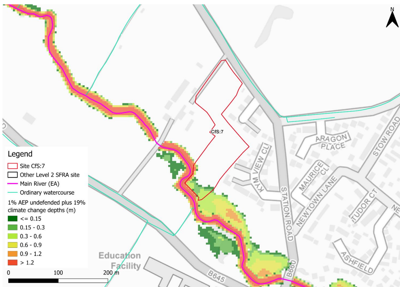
Figure 2-6: Flood depths for 1% AEP undefended flood event +19% (central climate change allowance)
