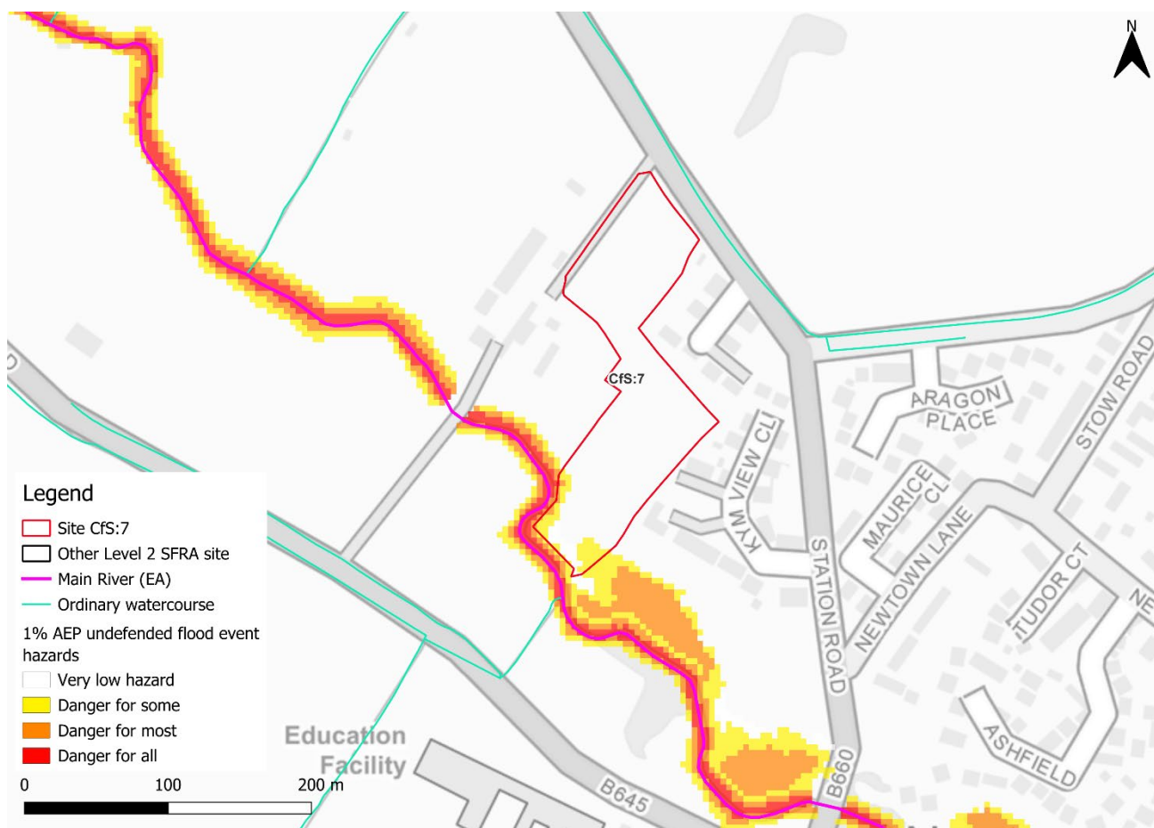
Figure 2-4: Flood hazard 1 for 1% AEP undefended flood event
