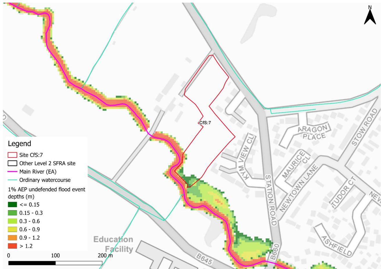
Figure 2-2: Flood depths for 1% AEP undefended flood event
