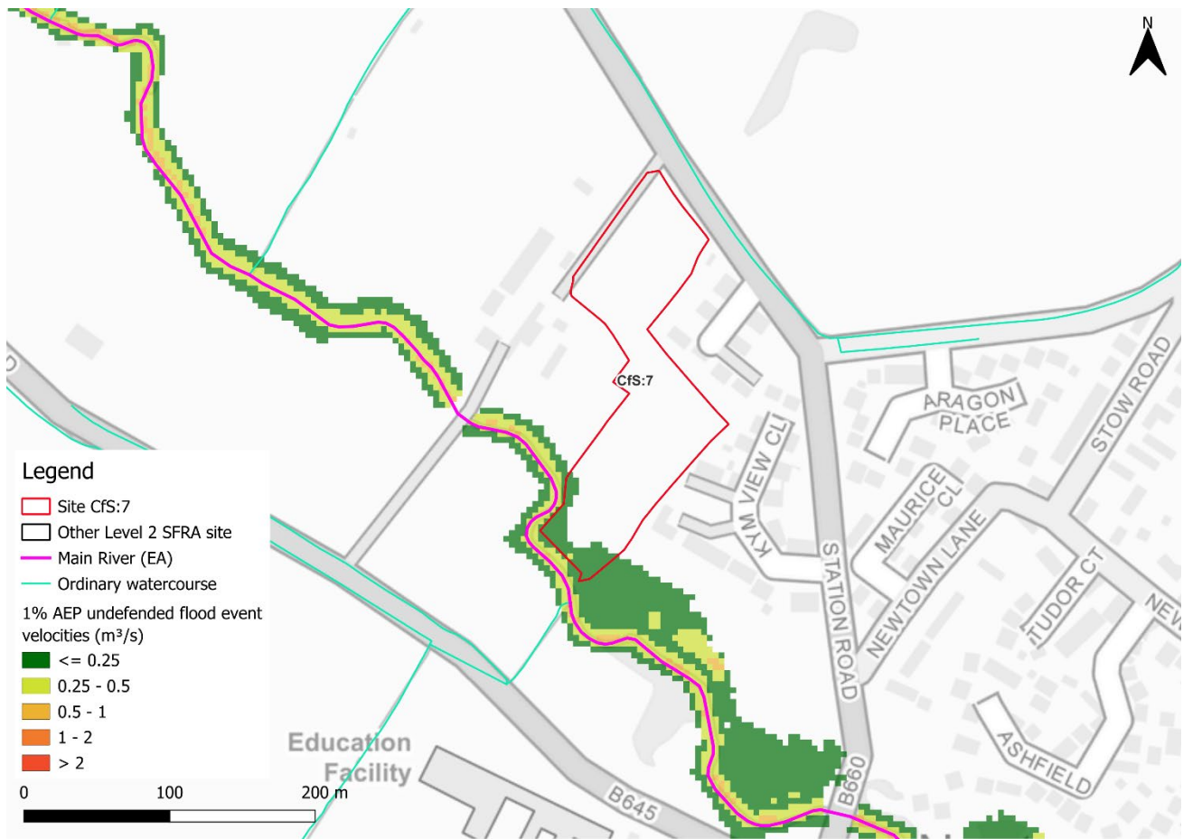
Figure 2-3: Flood velocities for 1% AEP undefended flood event
