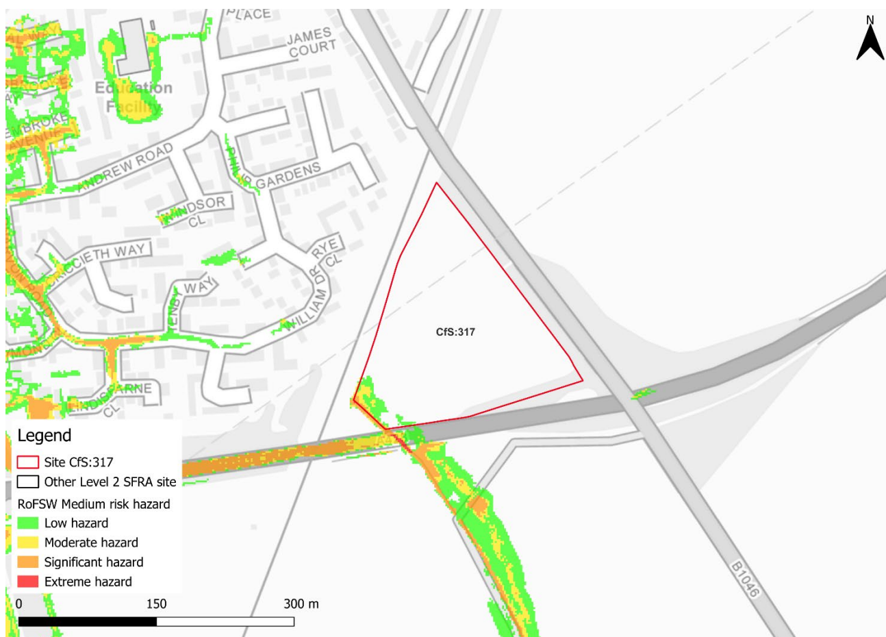
Figure 3-3: High risk event surface water flood hazard 1 (Third generation - Risk of Flooding from Surface Water map)
