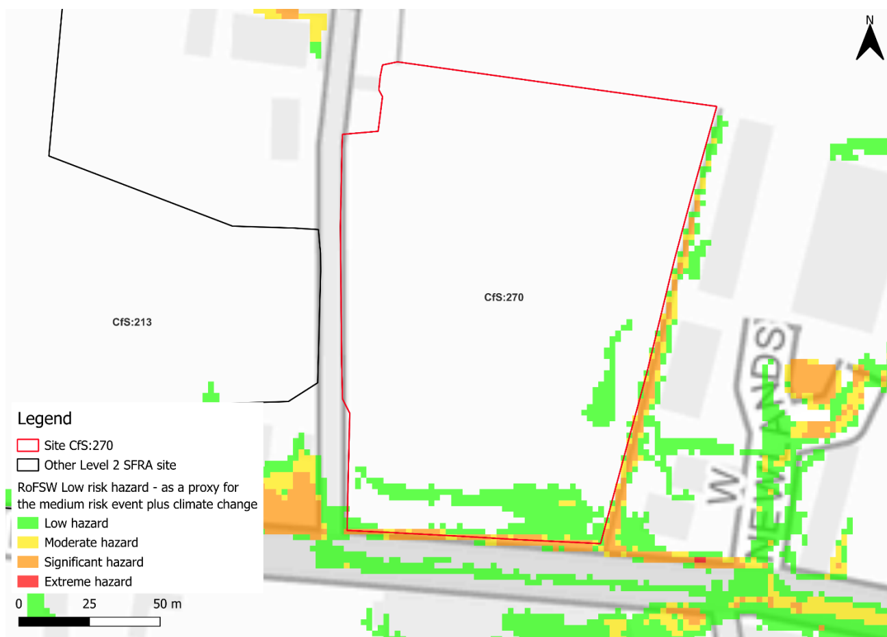
Figure 3-6: Low risk event surface water flood hazard, as a proxy for the medium risk event plus climate change (Third generation - Risk of Flooding from Surface Water map)
