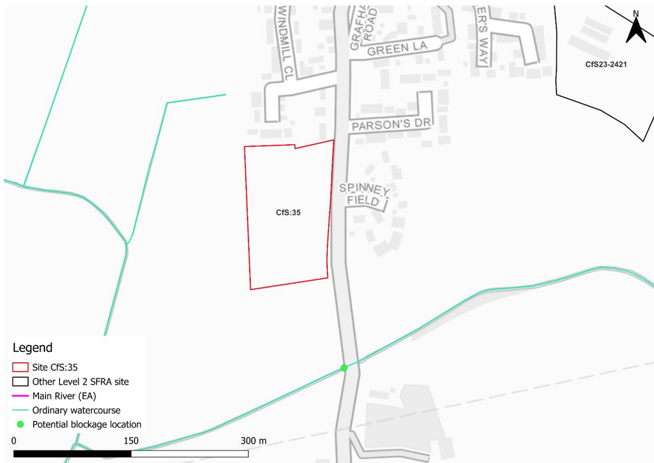
Figure 6-1: Potential blockage locations
