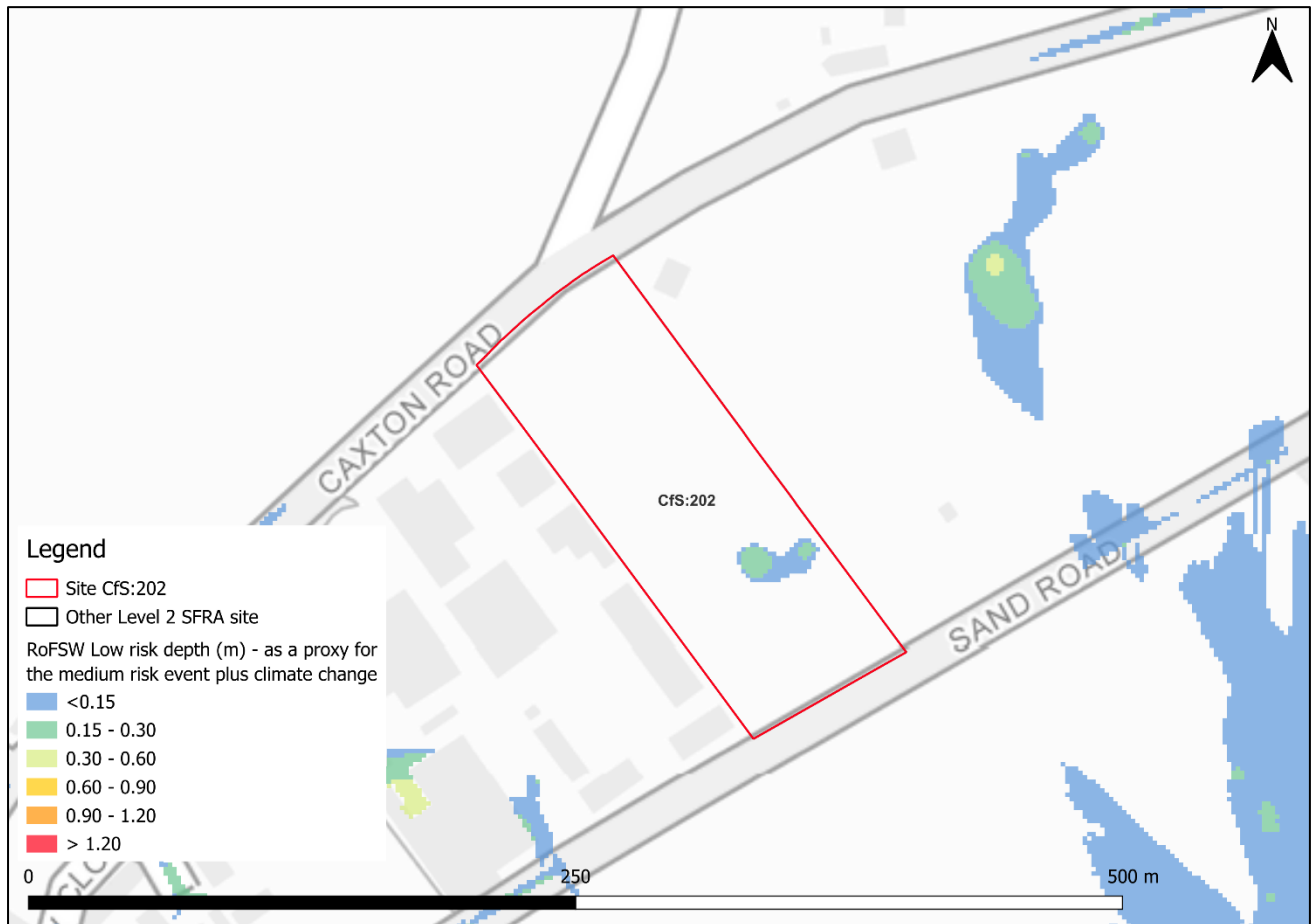
Figure 3-3: Low risk event surface water flood depths, as a proxy for the medium risk event plus climate change (Third generation - Risk of Flooding from Surface Water map)
