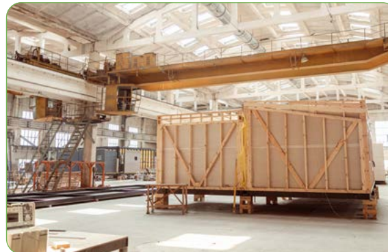
Composite wooden sip panels erected in a factory
