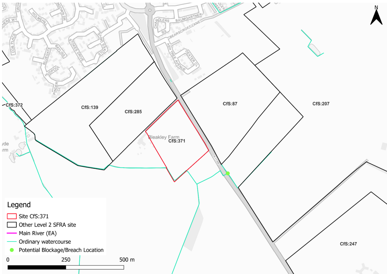
Figure 6-1: Potential blockage / breach locations
