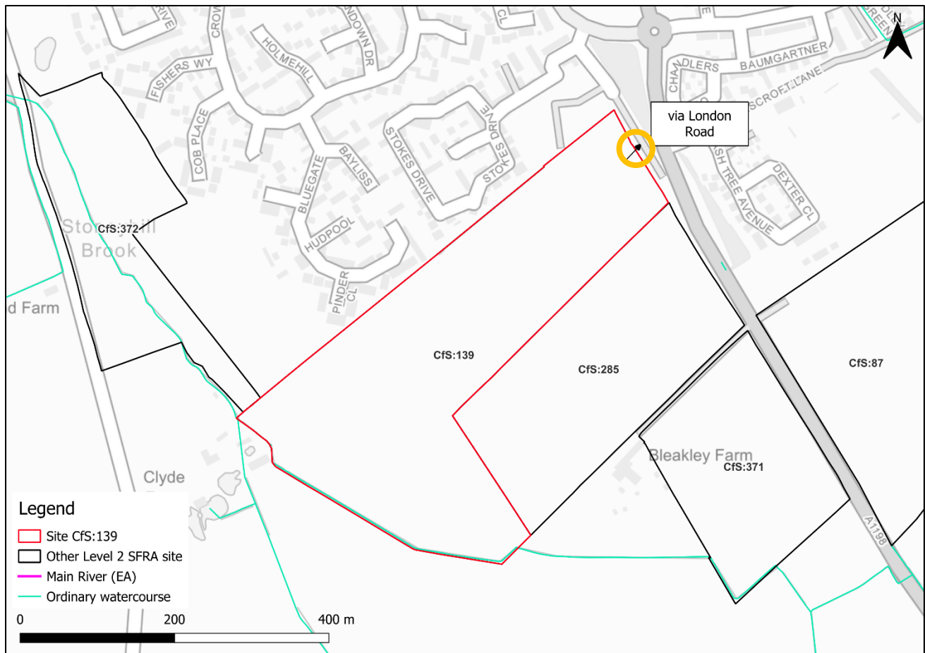
Figure 2-4: Potential access and escape routes
