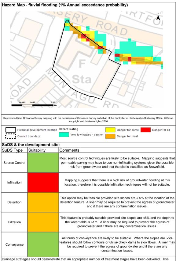
Drainage strategies should demonstrate that an appropriate number of treatment stages have been delivered. This depends on the factors such as the type of development, primary source of runoff and likelihood of contamination. Guidance should be sought from the LLFA and other guidance documents such as the CIRIA SuDS Manual (C753).
